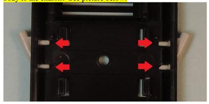
The body post receivers on the chassis may be chamfered using a countersink or a drill bit to allow for the free movement of the body posts. In addition, the ends of the body posts may also be slightly tapered to also allow for their free movement in the body posts in the body post receivers on the chassis. See pictures below:
